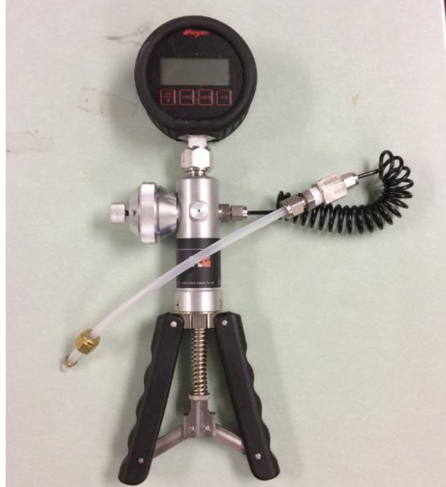
Figure 3.4. The combination of DPG-107 Dwyer digital pressure gauge and A T-970 Ametek pneumatic hand air calibration pump
